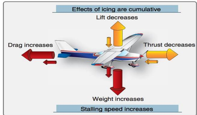
Figure 15-2. Effects of structural icing.
